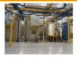
system guarantees, according to the customer expectations, fast color changes and permanent clean environment on the entire booth floor, avoiding powder accumulation and increasing the powder recovery up to 96%. The OptiCenter OC08 is equipped with OptiFlow IG07 injectors, that ensure precise and optimal powder feeding to the guns.
