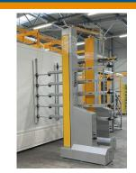
Kratki decided to purchase an automatic powder coating application for quick color change with a part contour scanning system from **Gema Switzerland**.
