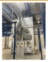
The vacuum floor of the manual stations keeps the workshop clean and the operators work in a less polluted environment. Energy savings have been made possible thanks to the frequency converter, which switches the filter to idle when parts are no longer passing through.
