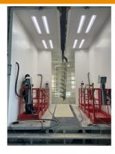
"Many production lines get stuck when processing complex constructions. To avoid this, we have doubled our hanging system. As a result, production speed remains constant and our production line is suitable for large as well as smaller and more complex objects. Our production speed is 33% faster than what we know from the market. In addition, we have increased the crossbars by 20% so that the maximum height is 3 meters instead of 2.5 meters."
