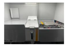
been equipped with the innovative OptiCenter All-In-One OC06 powder center, the first system that combines electrostatic control and powder transport via high-density venturi technology in a single unit.
