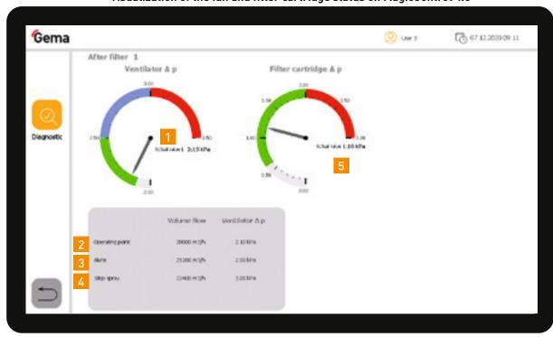
Visualization of the fan and filter cartridge status on MagicControl 4.0
