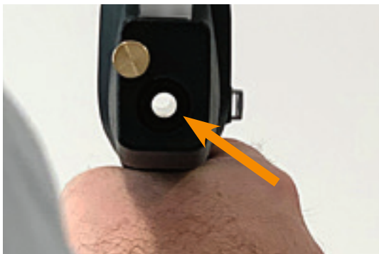
Visual check of the entire powder tube
