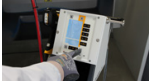
Step 4: Start the cleaning process
