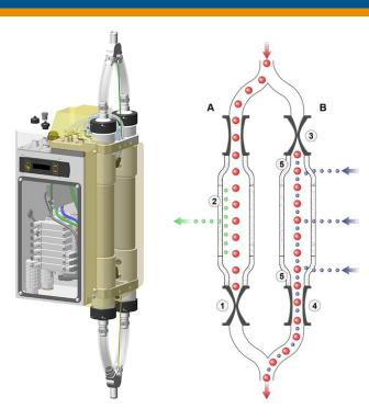
Step 2 – Transfer Transport air pushes powder from the alternate chamber to feed location
