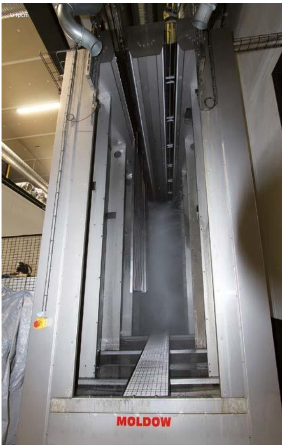
The exit of the seven-stage chemical pre-treatment spray tunnel and an example of the hanging solutions provided by HangOn.
