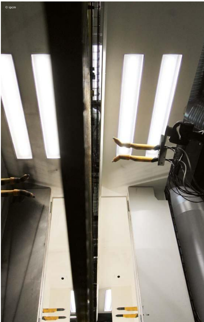
The touch-up robot in front on the coating booth.
