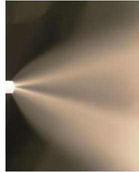
too much electrode rinsing air
