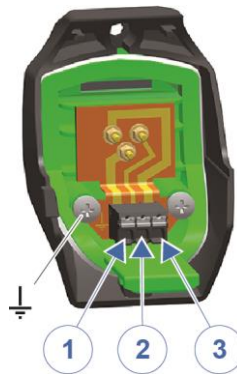
Fig. 13: Lid – Connections (cable numbers)
