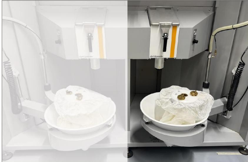
Fig. 97: Placing fresh powder - working area 2
