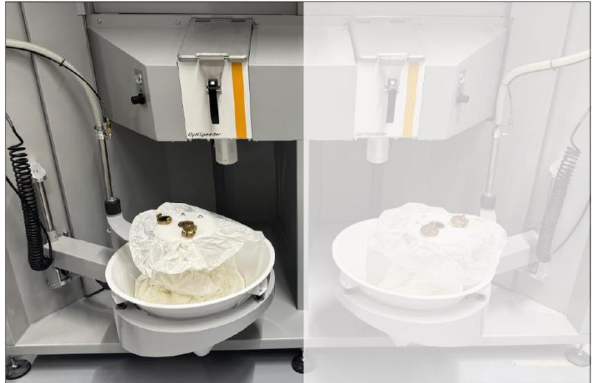
Fig. 96: Placing fresh powder - working area 1
