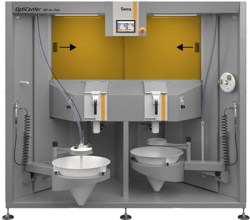
Fig. 9: Sliding doors (left/right)
