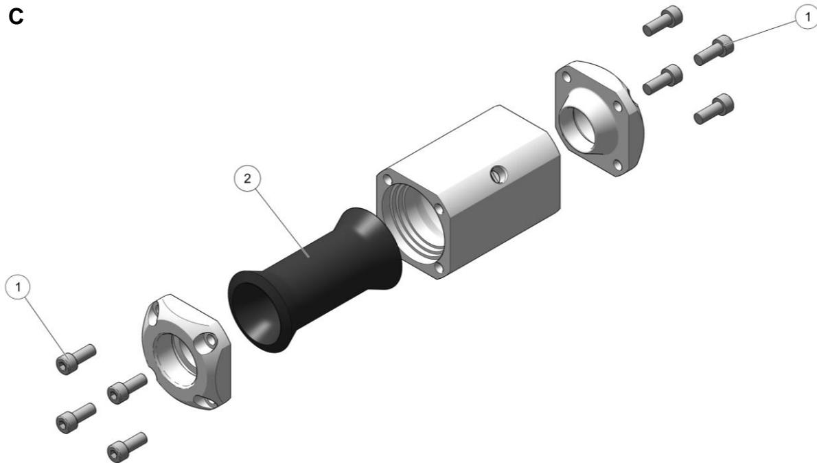
Fig. 114: Pinch valve D32 – complete
