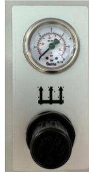
*Fig. 11: OptiSpeeder indicator fluidization*
