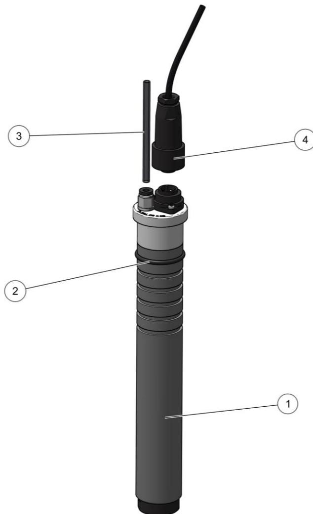
Fig. 122: LC01 Level sensor
