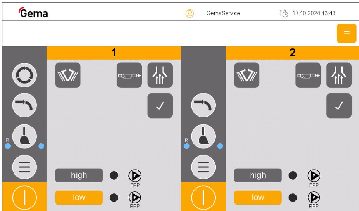
Fig. 87: Neutral state in “sequential” mode – ready for operation
