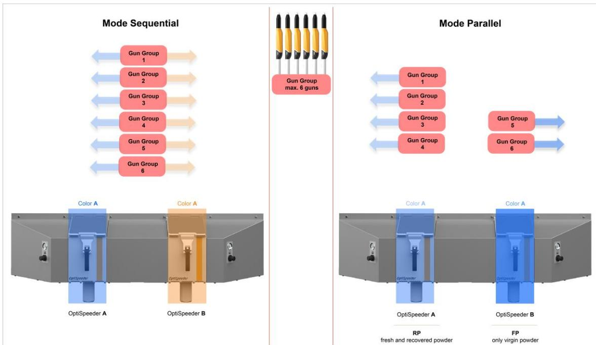
Fig. 21: Functional principle of gun grouping
