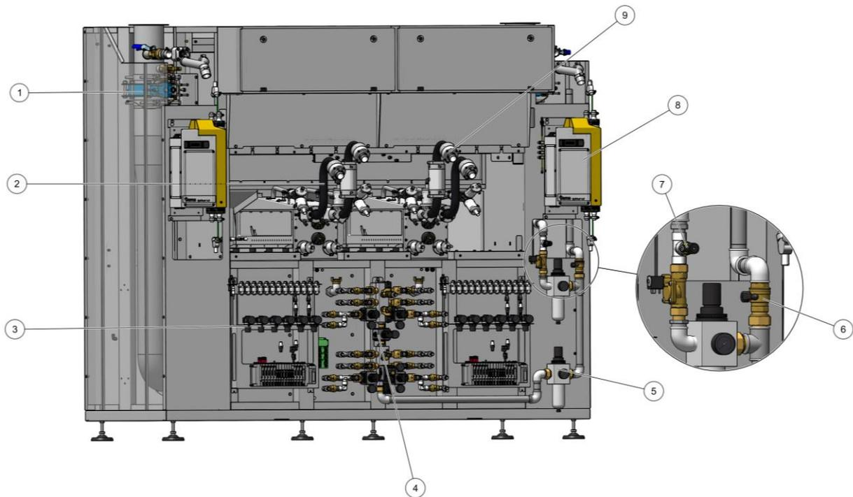
Fig. 108: OptiCenter – Pneumatics
