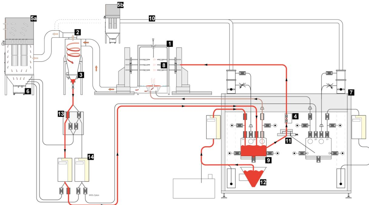
Fig. 28: Powder flow “Recycling”
